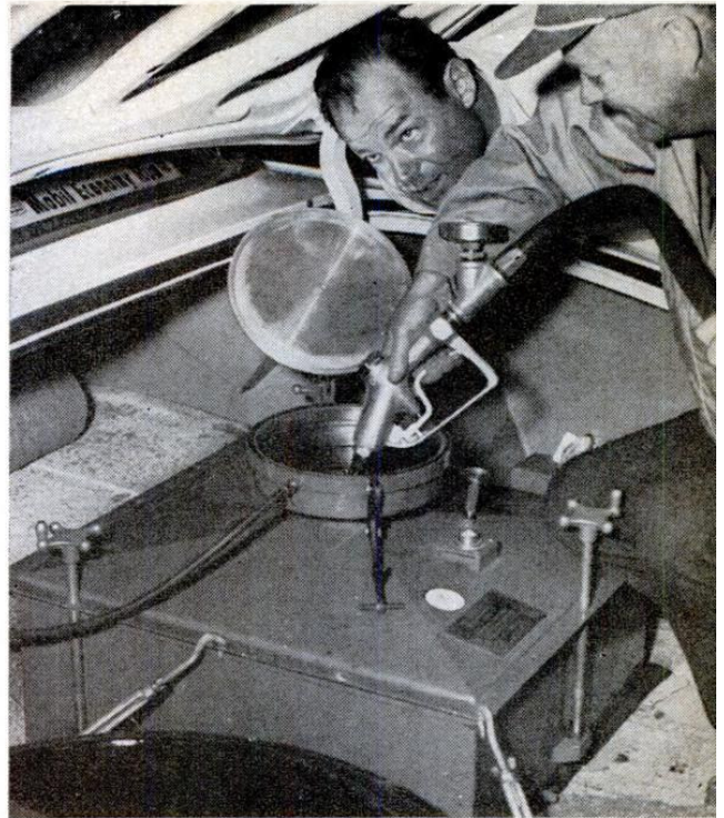
GASOLINE is metered into special Mobil Run tank by a U.S.A.C. official at two daily fuel stops. Gas is measured in 1/50th gallon increments at topoffs
